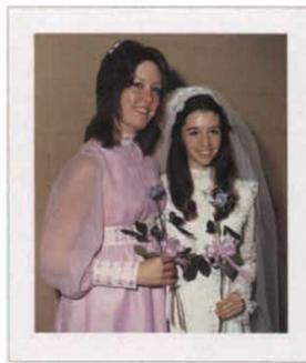
Fujicolor SFA3 print after 60 days in accelerated dark fading/staining test.
