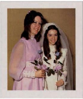
Fujicolor SFA3 print after 120 days in accelerated dark fading/staining test.
