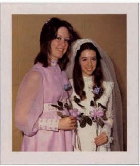
Fujicolor SFA3 print after 180 days in accelerated dark fading/staining test.
