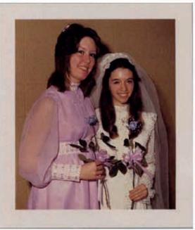
Fujicolor SFA3 print after 240 days in accelerated dark fading/staining test.
