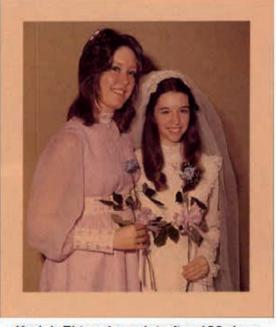
Kodak Ektacolor print after 180 days in accelerated dark fading/staining test.
