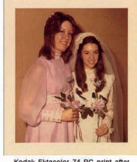
Kodak Ektacolor 74 RC print after 60 days in accelerated dark fading/dark staining test.
